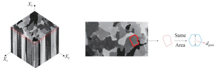
Figure 2 Polycrystalline ice's geometric structure and the method for equivalent crystal area
