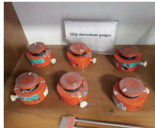
(b) Displacement sensors for capturing the motion data of the floating breakwater in the laboratory setup
