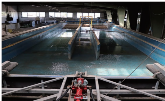
Figure 1 Wave flume setup at the SCWMRI hydraulic laboratory
