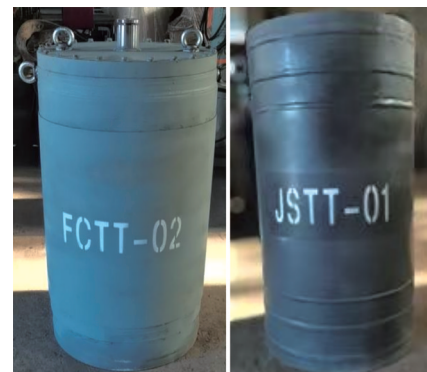
Figure 4 Physical models (Laminated model on the left, steel model on the right)
