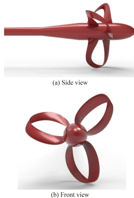
Figure 1 Geometry of the toroidal propeller model
