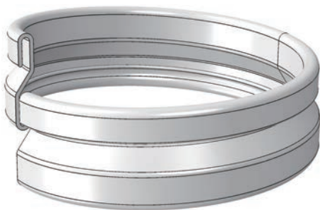
Figure 3 Three-dimensional model of the carcass layer ring
