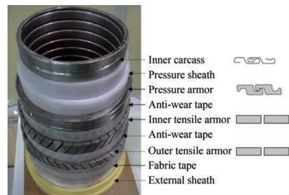
Figure 1 Structure of a typical flexible riser layer (Pinto and Gomes, 2017)
