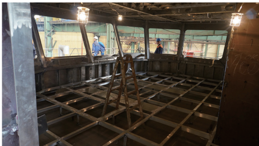
Figure 5 Picture of the frame supporting the floating floor taken during the construction
