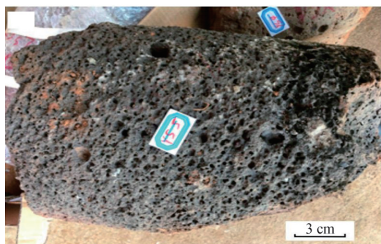
(b) Porous basaltic core samples from the yongshi farm site
