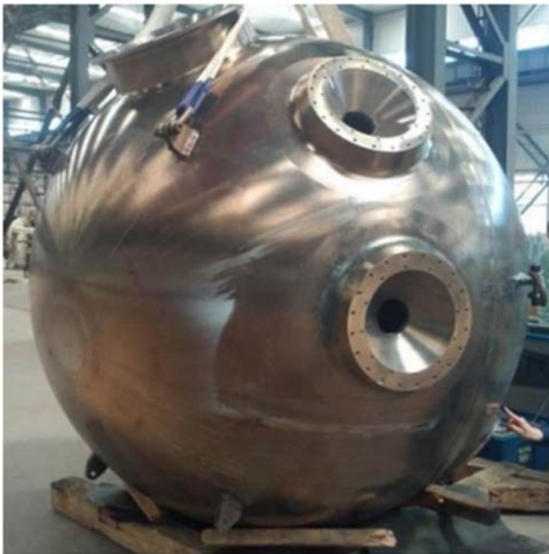
Figure 1 Spherical pressure hull of manned submersible, adopted by Li WY (Li et al. 2016)
