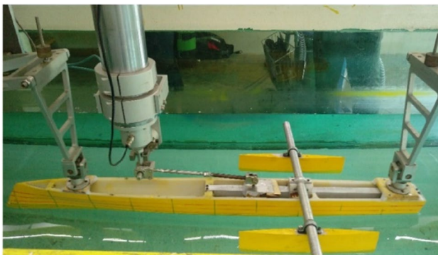
Figure 12 Experimental setup of National Iranian Marine Laboratory (NIMALA) towing tank
