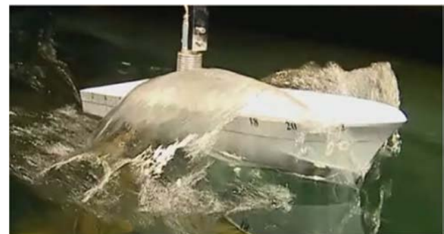
Figure 20 Bow wave spray from experiment at 14 kn
