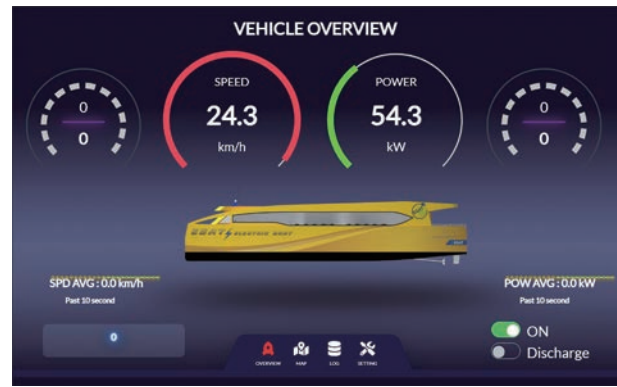
Figure 14 Monitoring Graphical User Interface of the electric-powered workboat
