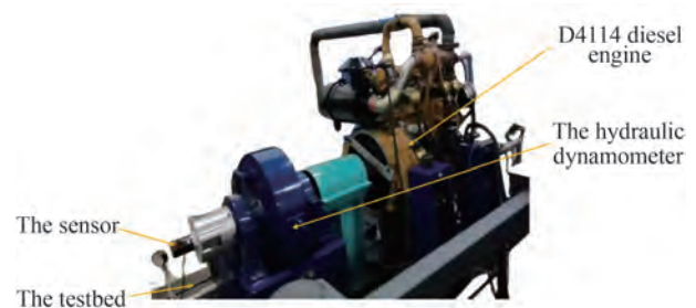
Figure 7 Test bench of D4114 marine diesel engine
