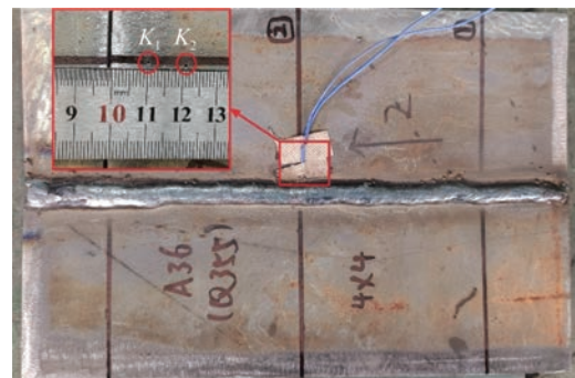
Figure 3 Experimental structure and temperature measurement points
