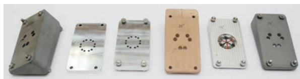
Figure 10 Wedges, from left to right: first, corresponds to \alpha = 5^\circ , \beta = 30^\circ , \gamma = 0^\circ ; then, variations are for angle \alpha only: 1.25^\circ , 2.5^\circ , 20^\circ , 5^\circ and 10^\circ
