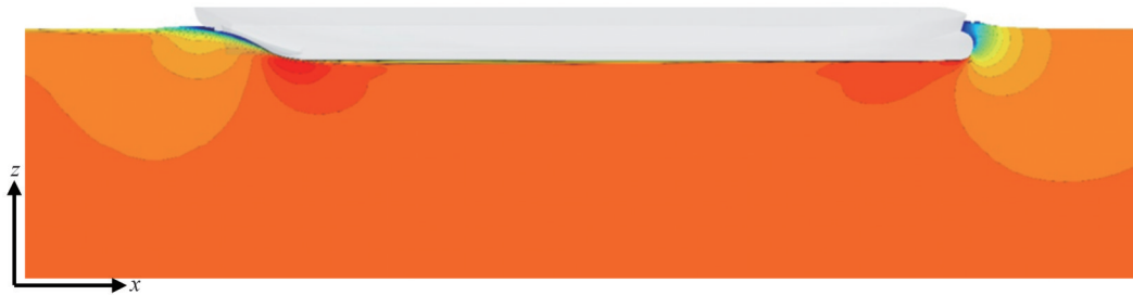
Figure 20 Velocity distribution in deep water ( H = 24T )
