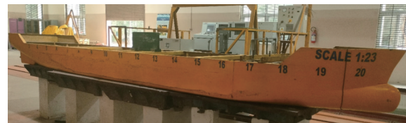
Figure 2 Model of the mini-bulk carrier
