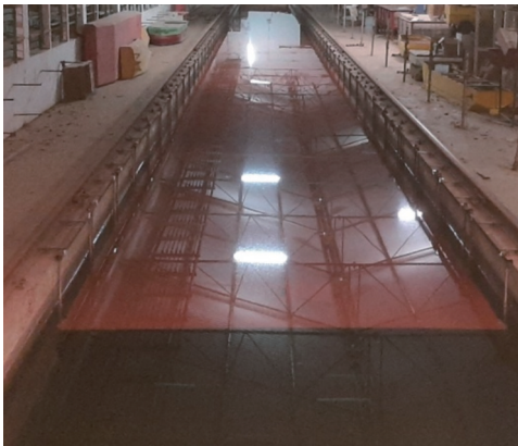
Figure 3 Shallow water towing tank
