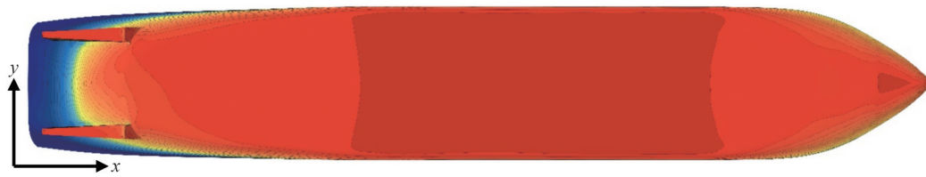
Figure 23 Pressure distribution on the hull surface in shallow water ( H = 2T )
