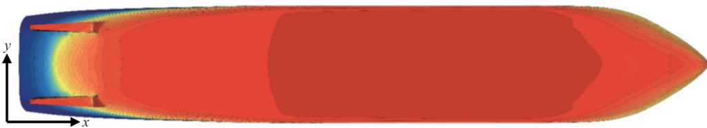
Figure 21 Pressure distribution in deep water ( H = 24T )
