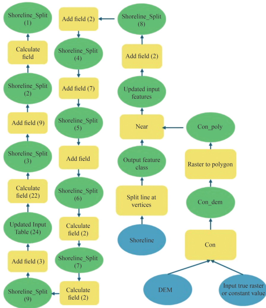
Figure 3 Visual representation of the ModelBuilder model constructed in ArcGIS software
