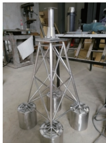
Figure 2 Test model of the four-bucket jacket foundation
