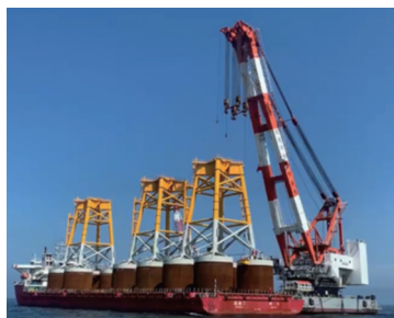
Figure 1 Jacket foundation of an offshore wind turbine
