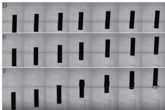
Figure 6 Image display of the vertical release cylinder water exit process
