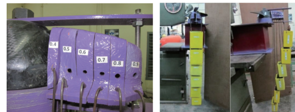
Figure 10 Segmented loading for static deflection analysis (Kumar et al., 2019)
