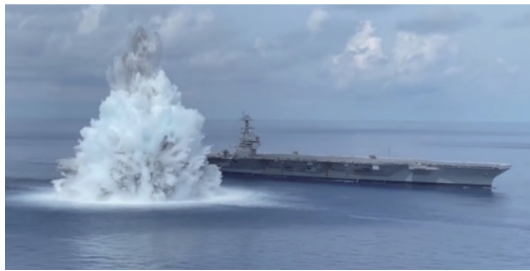
Figure 15 Marine explosion test on USS Gerald R. Ford (Gung, 2021)
