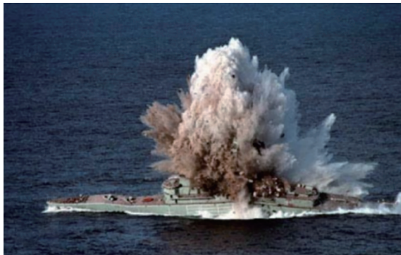
(a) Damage to ships caused by underwater explosions (Webster, 2007)
