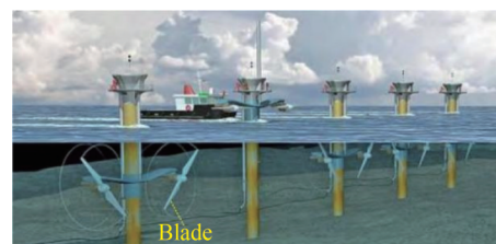
Figure 1 Concept of marine current turbine farm (Chen et al., 2018)
