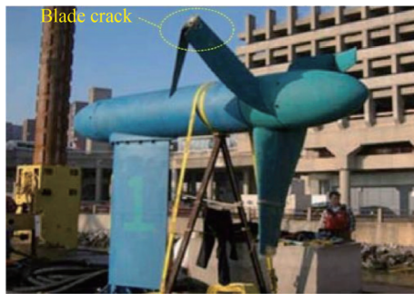
Figure 2 Picture of a blade crack in the actual engineering (Xie et al., 2020)
