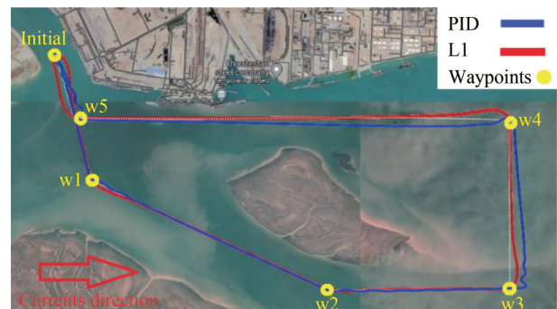
Figure 19 Trajectory of the vessel at the simulation of path-following in the geography map (Port of Bandar-e Emam Khomeyni)
