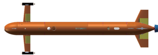
(a) AUV 1 (Flight-Style AUV with bow-wings)
