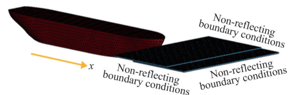
Figure 11 Schematic of the collision scenarios and boundary conditions between ships and rafted ice
