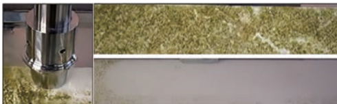
Figure 11 Ultrasonic cleaning device physical picture and cleaning before and after comparison (Mazue et al., 2011)
