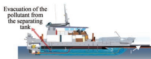
Figure 2 Principle underlying the ECOCEANE concept
