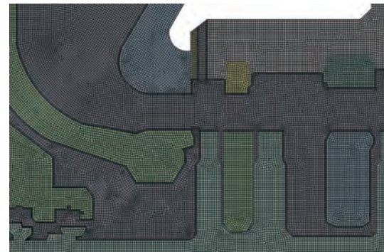
Figure 6 Discretized geometry of the turbine additional inlet
