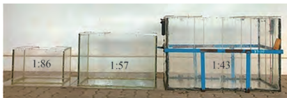
Figure 2 Photographic view of rectangular scaled tanks
