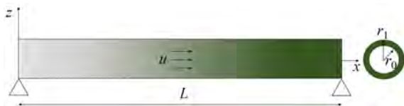
Figure 1 Schematic of an axially functionally graded material pipe
