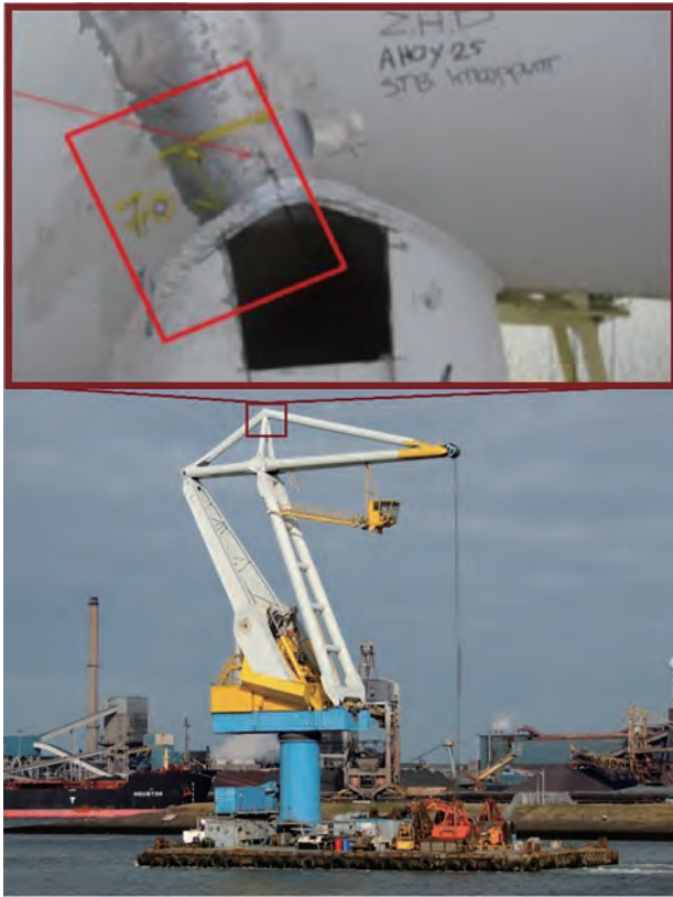
Figure 3 Crack propagation within upper arm joint of Cornelis Tromp 25T lemniscate crane
