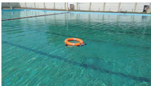
Figure 19 Prototype 3 overturned configuration testing in swimming Pool
