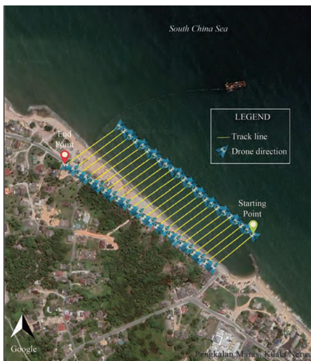
Figure 3 Flight lines for the auto-fly survey that have been planned in the Litchi application
