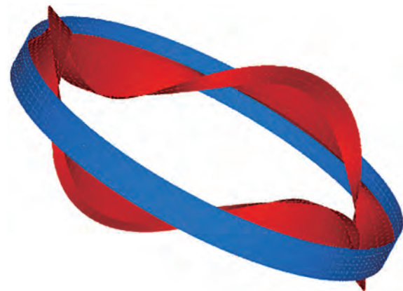
Figure 5 Buckling of the annular frame
