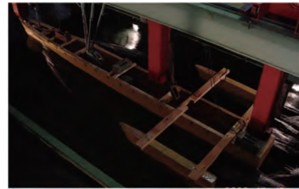
Figure 5 Model tests for Model A in the towing tank
