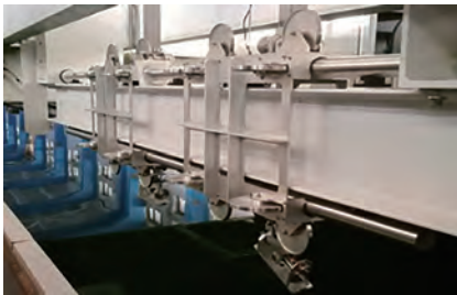
Figure 12 Four-component measuring instrument
