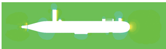
Figure 17 Pressure contours of the AUV self-propulsion with the designed propeller
