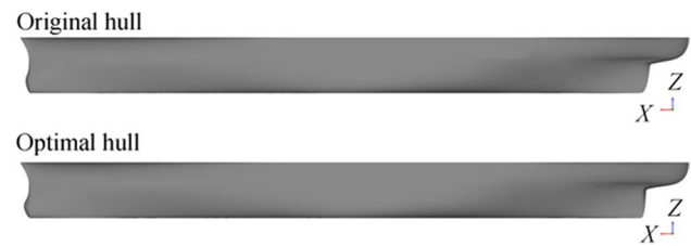
Figure 27 Comparison of the original hull and the optimal hull for the S-175 at Fr = 0.250
