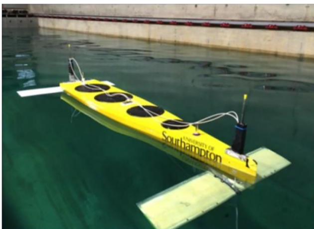
Figure 5 USV AutoNaut of the University of Southampton (Bowker et al. 2016)
