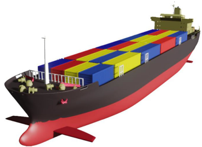
Figure 6 An artist's view of a container ship with energy-saving wings
