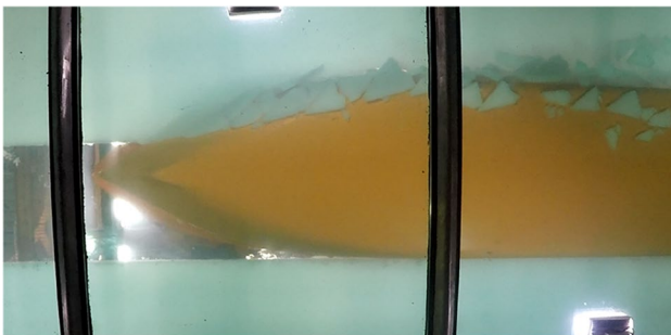
Figure 5 Model tests of large carrier ship in the ice channel free from broken ice. Asymmetric movement
