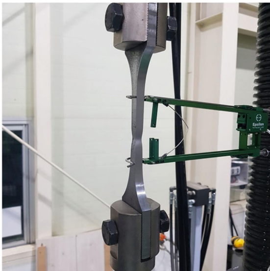
(b) Specimen with extensometer
