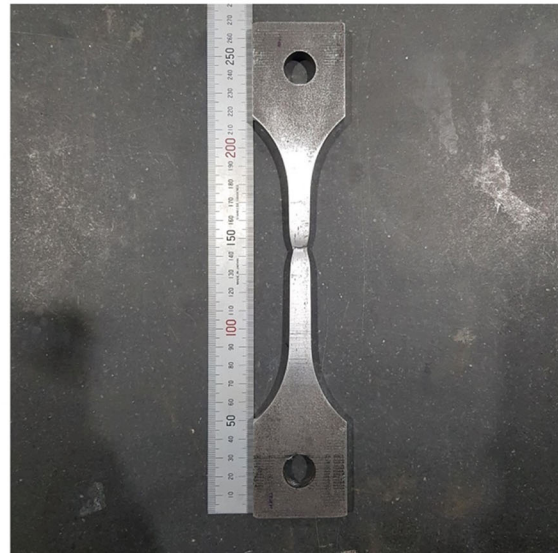
(c) Specimen after completing tensile test
