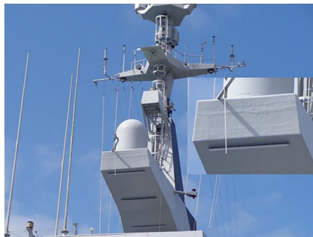
Figure 5 Naval ship top mast built up in fiberglass composite
