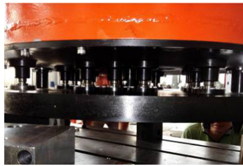
Figure 17 SCM after docking and locking
