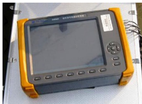
(a) Portable dynamic signal-testing analyzer
