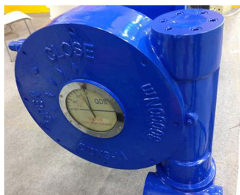
Figure 7 Position indicator on butterfly
