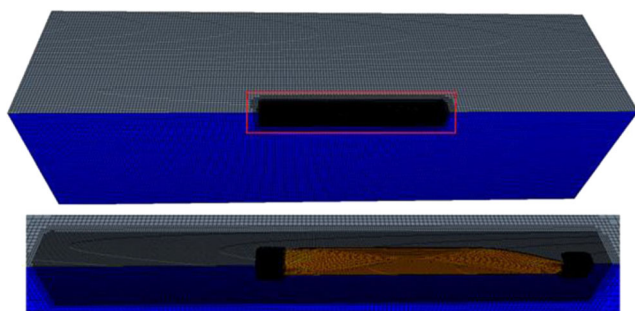
Figure 9 3D view of the KCS mesh
