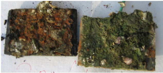
Fig. 3 Surface of the galvanically coupled coupons of 15CDV6 (left) & MDN250 (right) exposed in natural seawater
