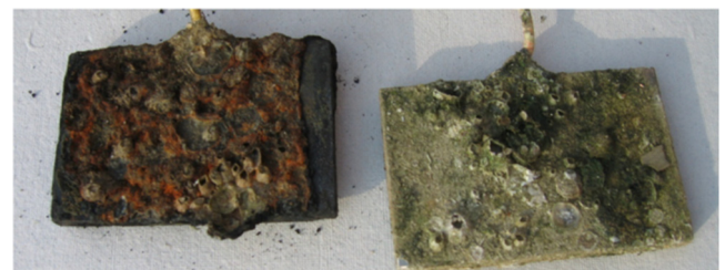
Fig. 5 Surface of the galvanically coupled coupons of 15CDV6 (left) & MDN138 (right) exposed in natural seawater
