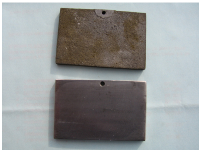
Fig. 6 Surface of the galvanically coupled coupons of 15CDV6 (top) & MDN138 (bottom) after removal of biomass and corrosion products
