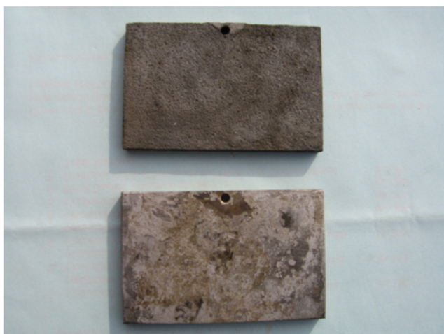
Fig. 4 Surface of the galvanically coupled coupons of 15CDV6 (top) & MDN250 (bottom) after removal of biomass and corrosion products
