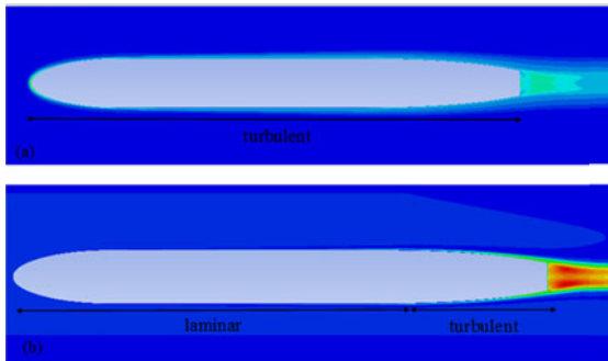
Fig. 7 Contours of turbulent kinetic energy; a) k-\epsilon turbulence model and b) Menter's SST-Transient model
