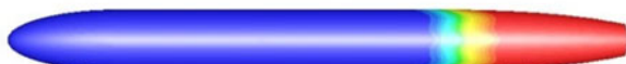
Fig. 8 Variations in intermency over the body surface, computed using Menter's SST-Transition model (laminar region, blue; turbulent region, red)
