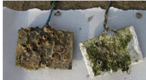
Fig. 4 Surface of the galvanically coupled coupons of HE15 (Right) & MDN138 (Left) exposed in natural seawater for 330 days
