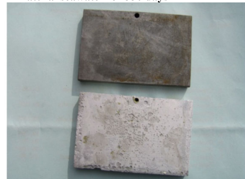
Fig. 5 Surface of the galvanically coupled coupons of HE15 (bottom) & MDN138 (top) after removal of biomass and corrosion products
