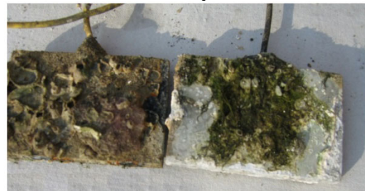
Fig. 6 Surface of the galvanically coupled coupons of HE15 (Right) & MDN250 (Left) exposed in natural seawater for 330 days
