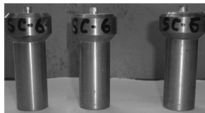
(b) Tools with cylindrical probes
