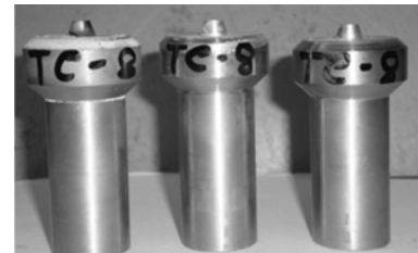
(c) Tools with tapered cylindrical probes
