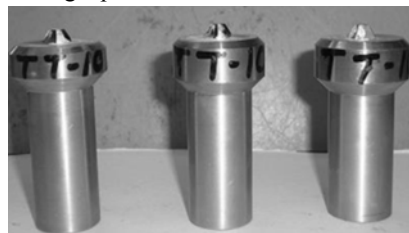
(a) Tools with trapezoidal probes
