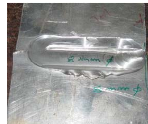
Fig.7 Limit setting of probe diameter for straight cylindrical tool
