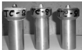
(c) Tools with tapered cylindrical probes
