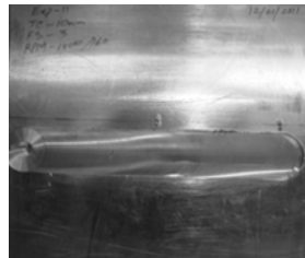
(a) Weld profile with straight cylindrical tool
