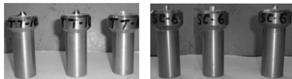
(a) Tools with trapezoidal probes; (b) Tools with cylindrical probes;
